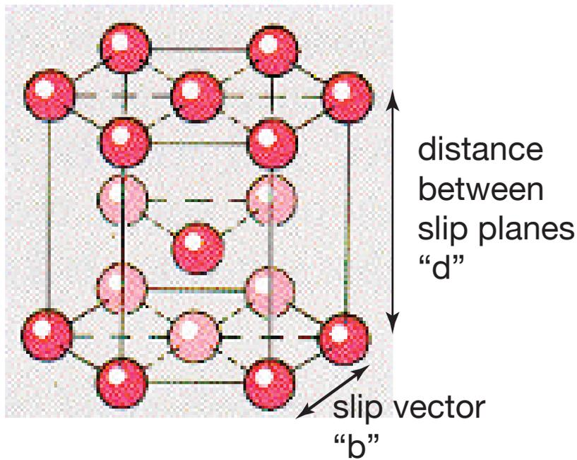
Slip is possible on different slip systems, meaning different combinations of slip-planes and slip directions.
